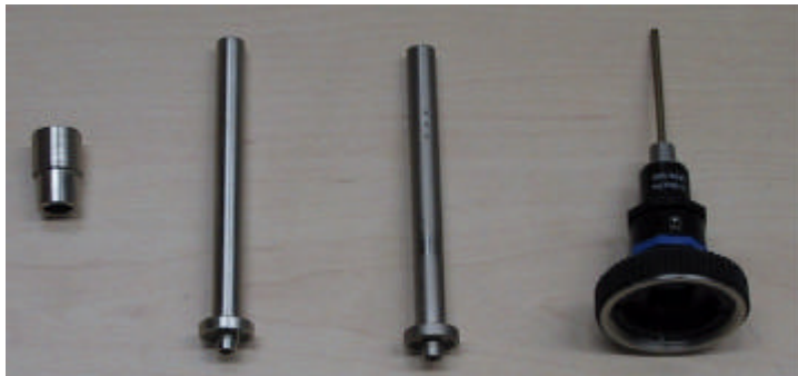
Figure 2. l.t.r. Beam attenuator, Open beam pipe, Half beam pipe, Half beam absorber
